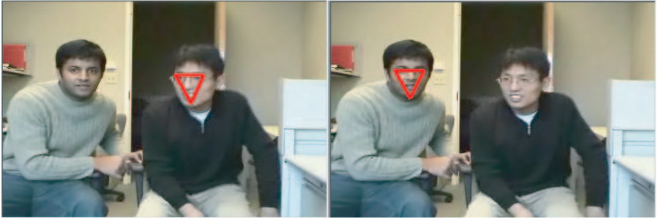
Figure 6: Tracking results in two consecutive frames on a sequence with two faces. Since the current tracking model assumes a single face, it occasionally jumps from one face to another when the (normalized) likelihood of a detection dominates in the MAP estimation of the pose.
