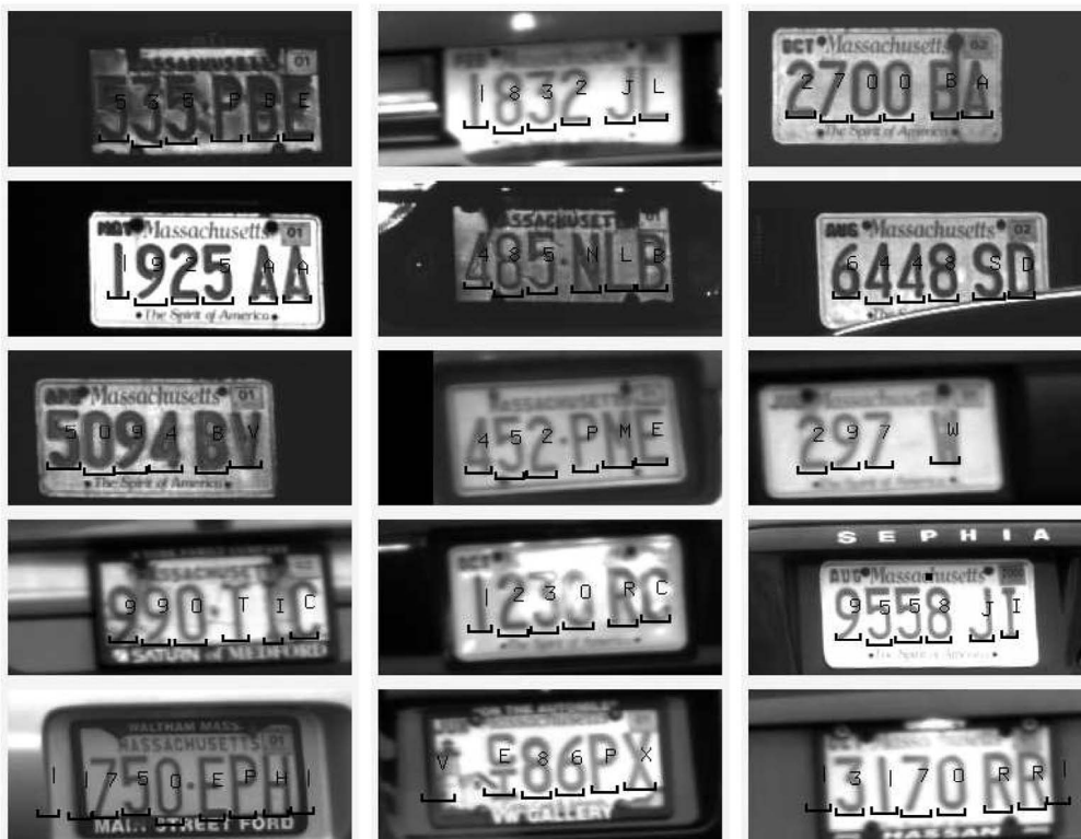
Fig. 11. Examples of detections on a variety of plates. The last row illustrates false positives.
